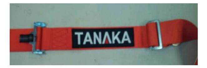
CAMS have been advised by the SFI Foundation Inc. of a recall of Driver Restraint Assemblies (safety harness) sold with the 'TANAKA' brand, and manufactured by Ruian Dragon. These safety harnesses carry the SFI 16.1 standard label.
